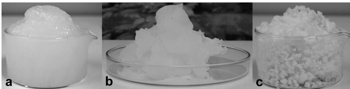
Figure 1. Used raw materials: (a) CNF, (b) TEMPO-oxidized fibers, and (c) BLWF.
